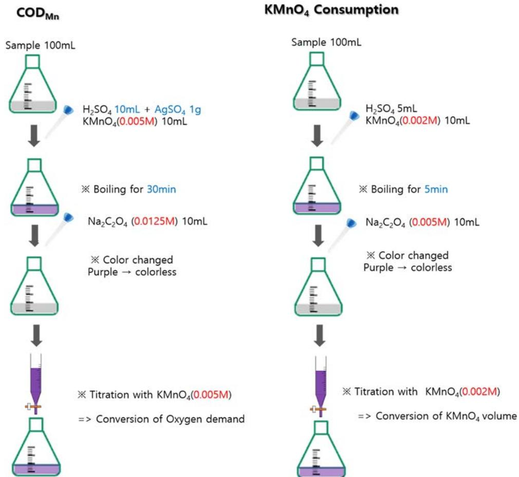
Figure 1. Analysis Process of  $\text{COD}_{\text{Mn}}$  and  $\text{KMnO}_4$  Consumption
